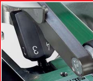
Adjustment of welding force for different materials
