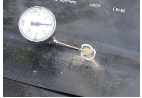
Testing of a welding seam with testing unit and injector needle.
