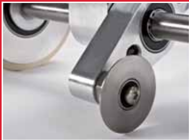
The guide roller holds the TAPEMAT on course.
